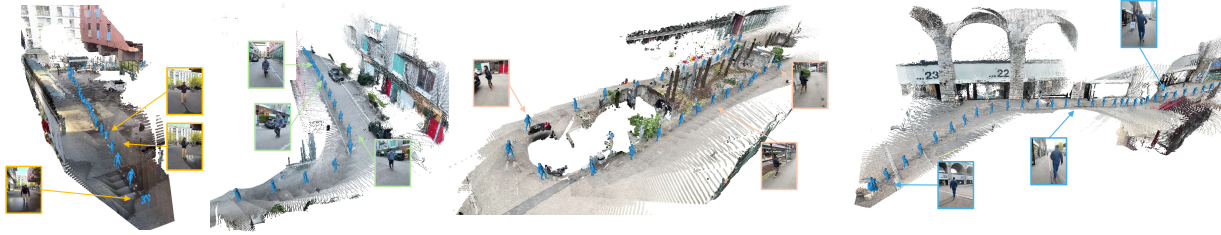
Fig. 7. Quality results of proposed 4D Human & Scene Reconstruction pipeline on EMDB dataset.
