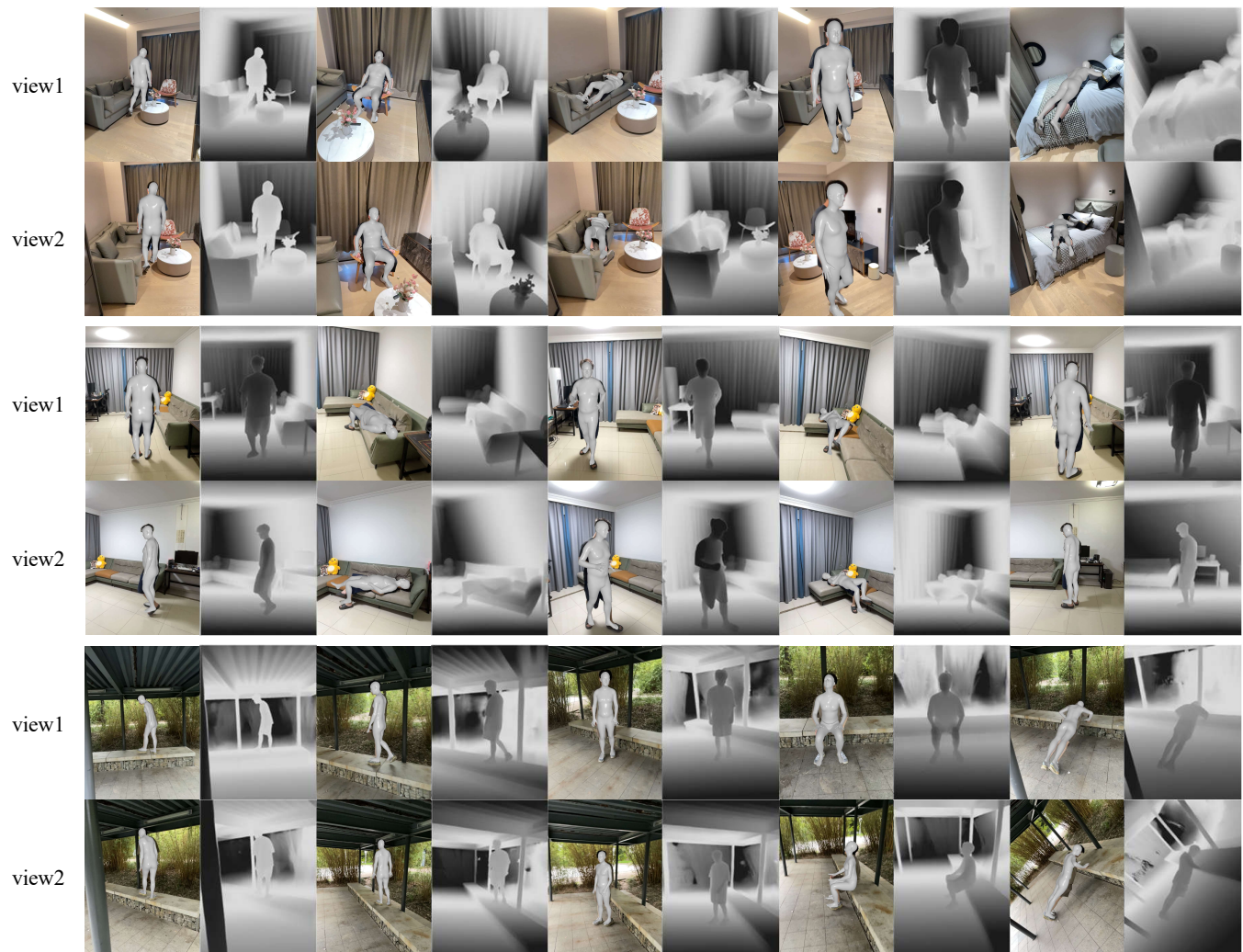
Fig. 11. Rendered SMPL and depth images of the captured dataset in camera space.
